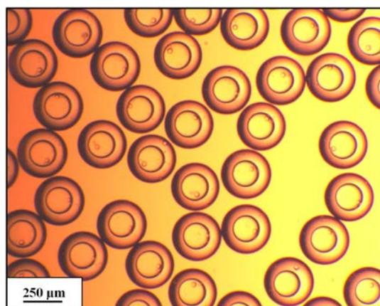
**Figure 1.** Optical microscopy image of a water-in PDMS-in water double emulsion.
