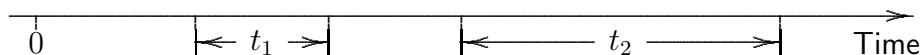
Figure 3.3: When deriving the Poisson process, we consider arrivals within two non-overlapping time intervals of duration t_1 and t_2 , respectively.
