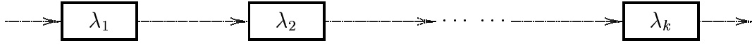
Figure 2.4: By combining k exponential distributions in series we get a steep distribution with formfactor \varepsilon \leq 2 ). If all k distributions are identical ( \lambda_i = \lambda ), then we get an Erlang- k distribution.
