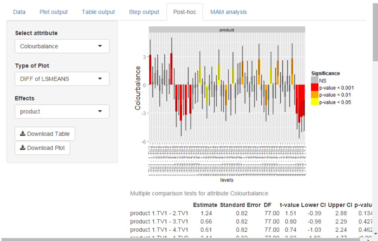
Figure 8: Screenshot for the post-hoc output for the Colourbalance attribute for the TVbo data
