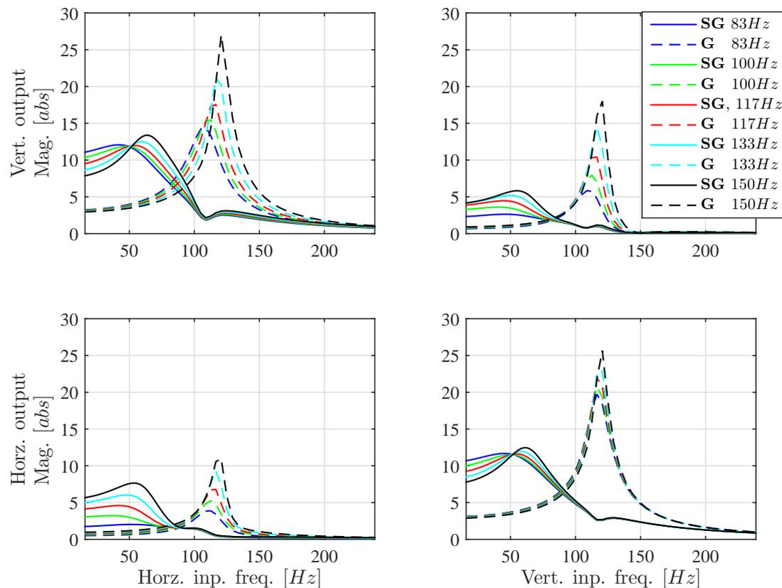
**Figure 5.** Evaluation of open and closed loop input disturbance responses ( $\mathbf{G}$ ,  $\mathbf{SG}$ ) for different rotation speeds extrapolated with the LPV model. The model shows, that the controller reduce the peak gain significantly.
