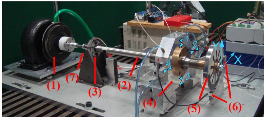
**Figure 1.** The experimental controllable gas bearing setup. A turbine (1) drives a flexible shaft (2), which is supported by both a ball bearing (3) and the controllable gas bearing (4) with four piezoactuated injectors. A disc (5) is mounted in one end to pre-load the journal and displacement sensors (6) measure the lateral movement of the disc in the shown reference frame. A quadrature encoder (7) measures the angular position.
