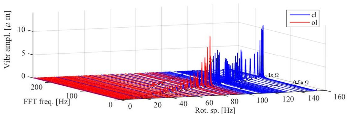
**Figure 7.** Waterfall diagram for vertical shaft direction to investigate the frequency content of the vibrations. In open loop (ol) the synchronous vibrations grow fast as the critical speed is approached. In closed loop (cl), the vibrations are sufficiently attenuated to allow faster rotation speeds.
