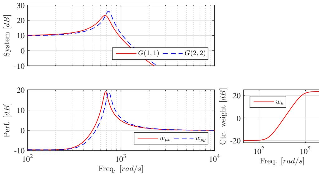
**Figure 3.** System gain, performance weights  $w_{px}(s)$ ,  $w_{py}(s)$  as defined in Eq. (11) and controller sensitivity weight  $w_u(s)$  as defined in Eq. (12). The two left plots share the frequency axis to show the performance weight peaks coincide with the natural frequencies.
