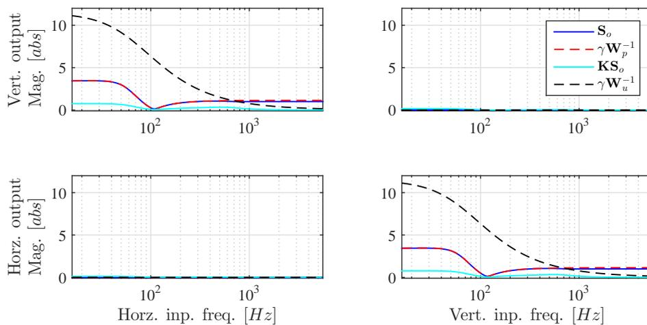
**Figure 4.** Resulting sensitivity functions  $\mathbf{S}$  and  $\mathbf{KS}$  and corresponding inverse scaled weights  $\gamma\mathbf{W}_p^{-1}$  and  $\gamma\mathbf{W}_u^{-1}$ . At low frequency, the performance closely follows the performance weight.
