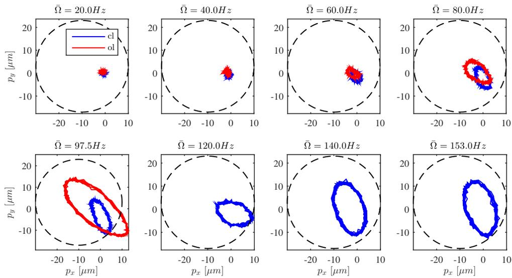
**Figure 6.** Experimental measurements for various shaft rotation speeds. In open loop (ol), the vibrations exceed the limit of safe operation at  $\Omega = 94.8 \text{ Hz}$ . In closed loop (cl), the control reduces the vibrations and significantly increases this limit.
