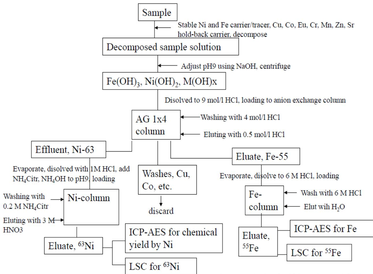
Fig. 2 Analytical procedure for determination of  $^{63}\text{Ni}$  and  $^{55}\text{Fe}$  using combined techniques of precipitation, ion exchange chromatography and extraction chromatography (Hou, et al. 2005)
