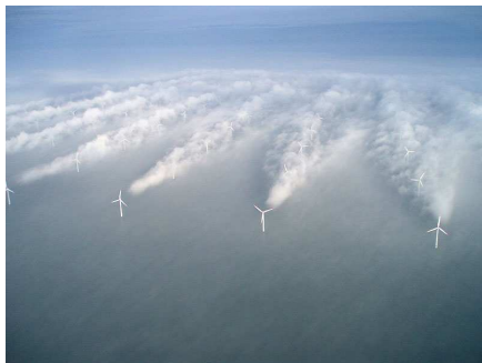
Wake effects in Horns Rev 1. Photographer Christian Steiness.
