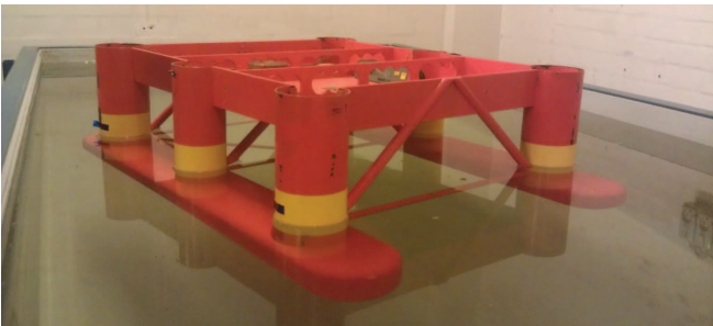
(b) Model-version of the semi-submersible (hull structure only).
