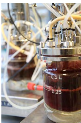
Batch cultivation of T. atroroseus at pH 5
