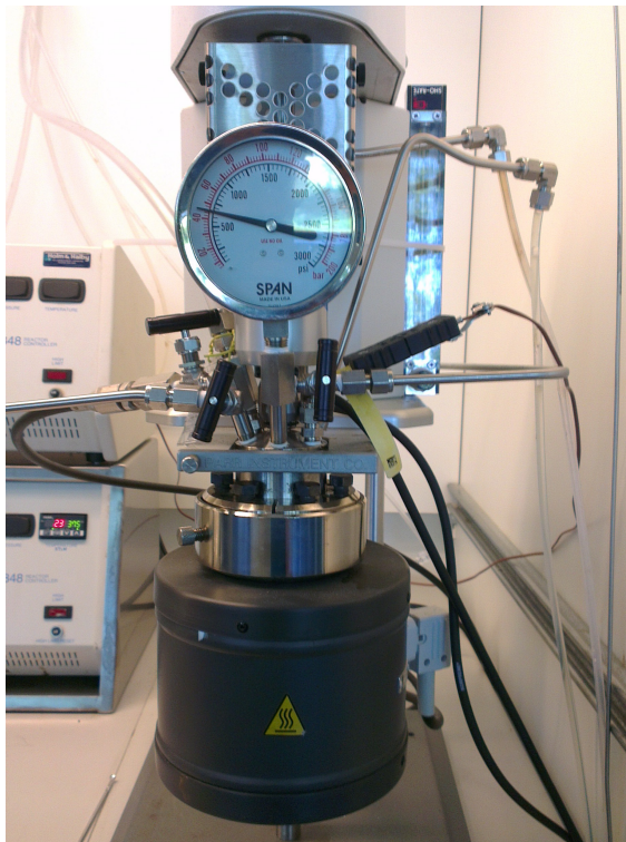
(a) Assembled batch reactor setup.
