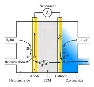
This work aims at investigation and improvement of existing FC research platforms by tuning catalysts for the Oxygen Reduction Reaction (*ORR*) for Proton Exchange Membrane (*PEM*) FCs applications. The overall project aims at identifying catalysts for High Temperature (*HT*) PEMFCs, which are resilient towards the phosphate anion poisoning associated with PolyBenzImadazole (*PBI*) based PEMs.
