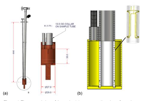
**Figure 1**. The general view of the probe (a), cross-section view of a probe including RF coil (b)
