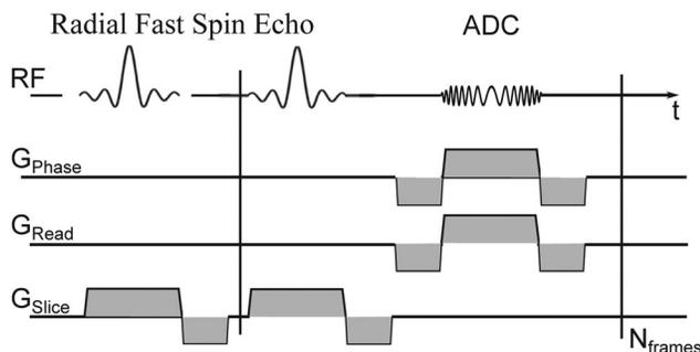
FIG. 1. A pulse sequence illustration of the radial 2D FSE sequence, with slice selective excitation and refocusing pulses. The radial angle scheme used was the golden ratio of  $111.25^\circ$  ensuring high temporal k-space coverage allowing time resolved images to be reconstructed.
