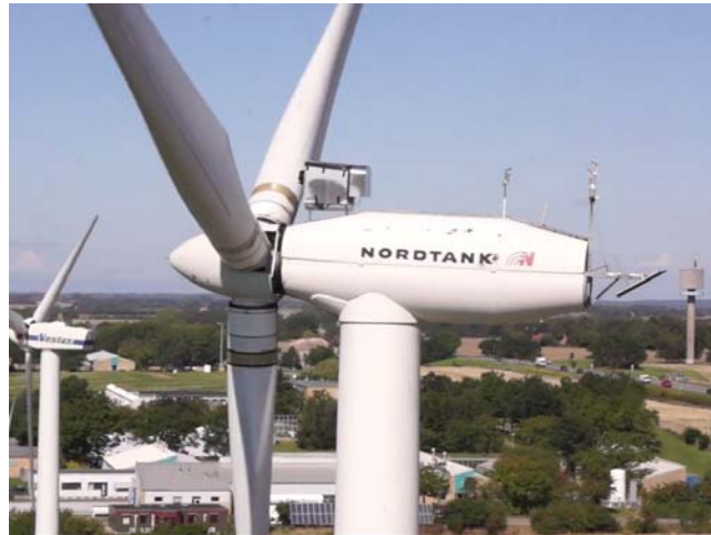
Figure 13: The SpinnerLidar installed on top of the NordTank turbine at DTU Risø campus.
