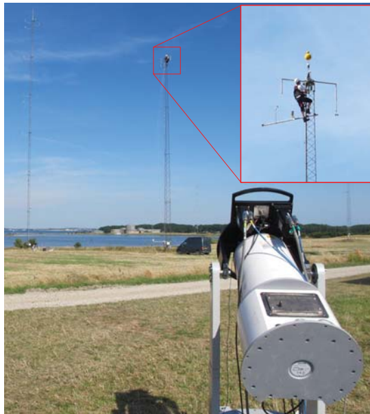
Figure 8: Photo of the one of the short-range WindScanners used (R2D2) and of the short met mast. The rotating ball installed on the short met mast appears to the right.
