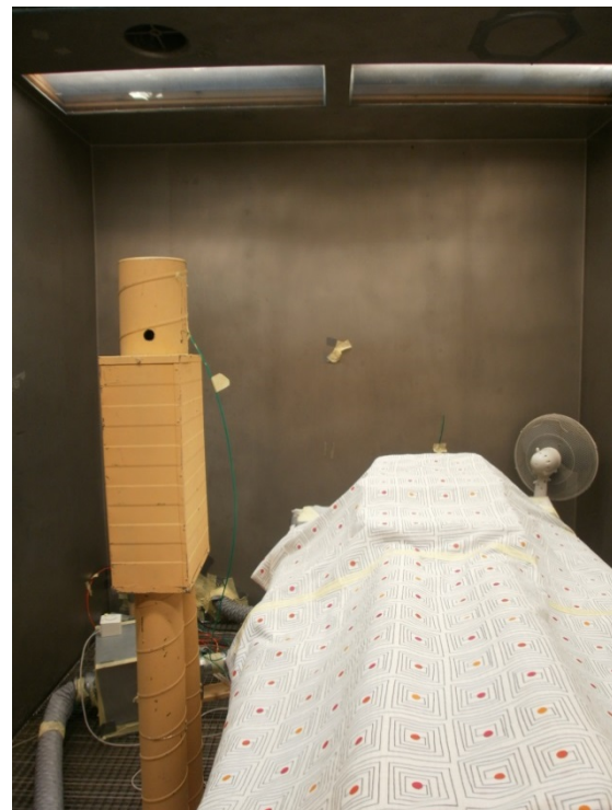
Figure 2. Experimental setup: (left) floor plan of the chamber showing the position of the sample tubes (*), where 1 – “doctor”, 2 – “lying patient” on a bed, 3 – total exhaust opening; (right) interior of the chamber with the standing dummy next to the bed with the ventilated mattress and the lying dummy on it.
