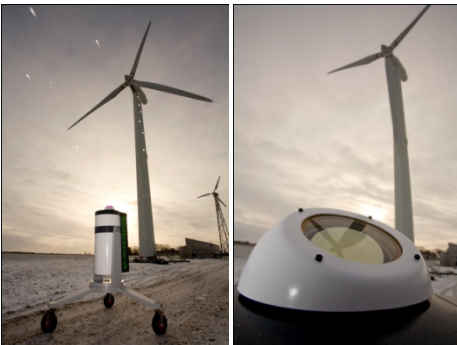
Figure 3. Left: Short-range prism-based half-sky ( \pi Sr) scanhead jointly developed by DTU Wind Energy IPU - Natural Power. Right: WindScanner R2D1.
