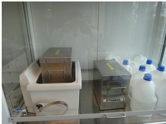
Figure 4.16: Acetone and ethanol tubs. Left: Acetone tub in ultra-sonic machine. Right: Ethanol tub.
