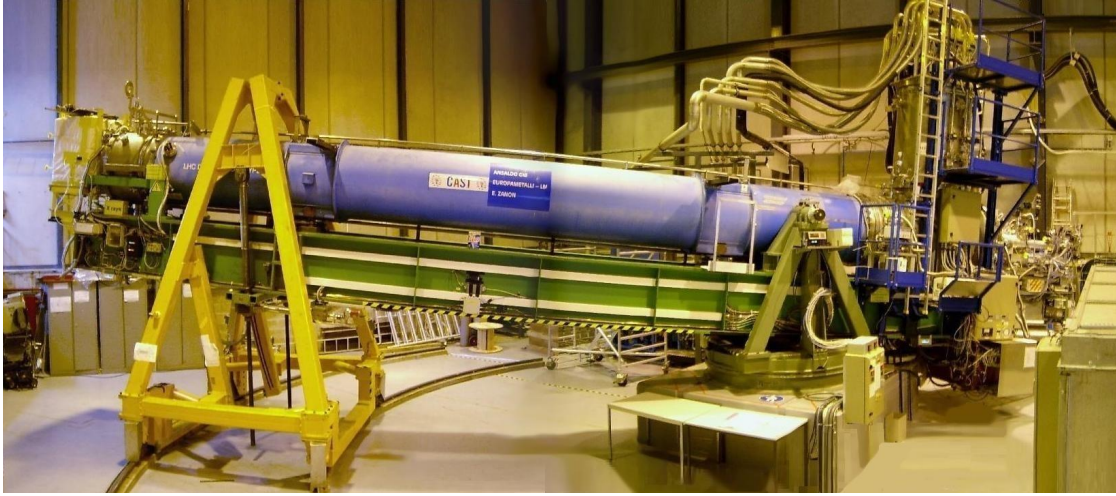
Figure 4.3: The Cern Axion Solar Telescope (CAST) located near Geneva, Switzerland. The main component of the experiment is a Large Hadron Collider (LHC) prototype dipole magnet that has a 10 T magnetic field, physical length of 13 meters and a mass of 50 tonnes.
