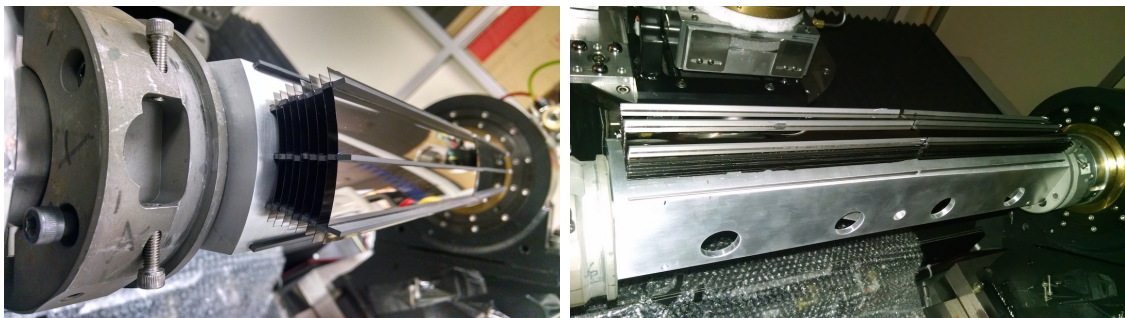
Figure 4.27: Pictures of glass substrates mounted on Ti mandrel during assembly. Three graphite spacers are attached on top of each glass substrate and machined to correct thickness before mounting of the next substrate.
