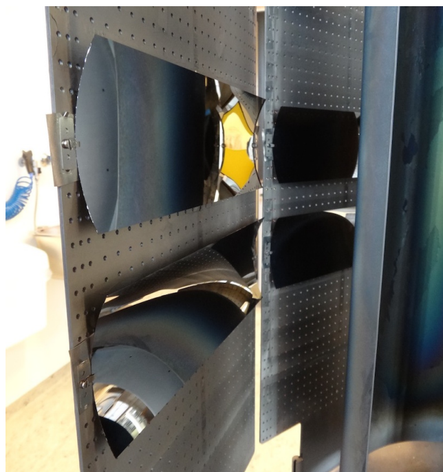
Figure 4.18: Mounted glass substrates in coating chamber after coating.
