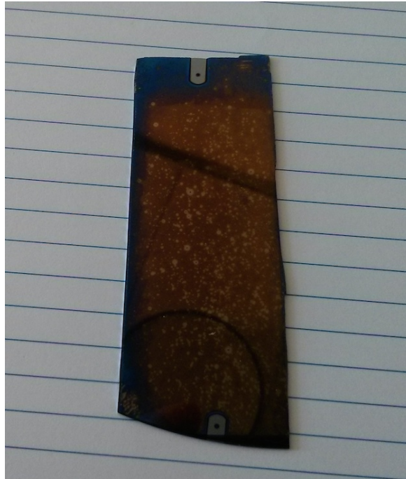
Figure 3.22: Picture of Si wafer sample coated with 10 bilayers of W/B 4 C using nitrogen reactive sputtering. Sample was coated in February 2012, picture taken July 2014. The surface over time turned a yellow/brown colour with the edges black/blue. Top and bottom are marks from the clips holding the sample in place during coating. The clear uncoated surface is visible in those spots.
