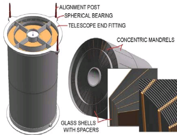
Figure 1.5: Illustration of an assembled NuSTAR optic. A central mandrel made from SiC is used as a base on which the first glass layer is attached to graphite spacers with epoxy. Each subsequent layer is attached using graphite spacers, resulting in a rigid construction. From [6]
