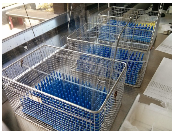
Figure 4.14: Glass substrates selected for the CAST XRT before cleaning. The substrates required for each recipe were collected in four different baskets.
