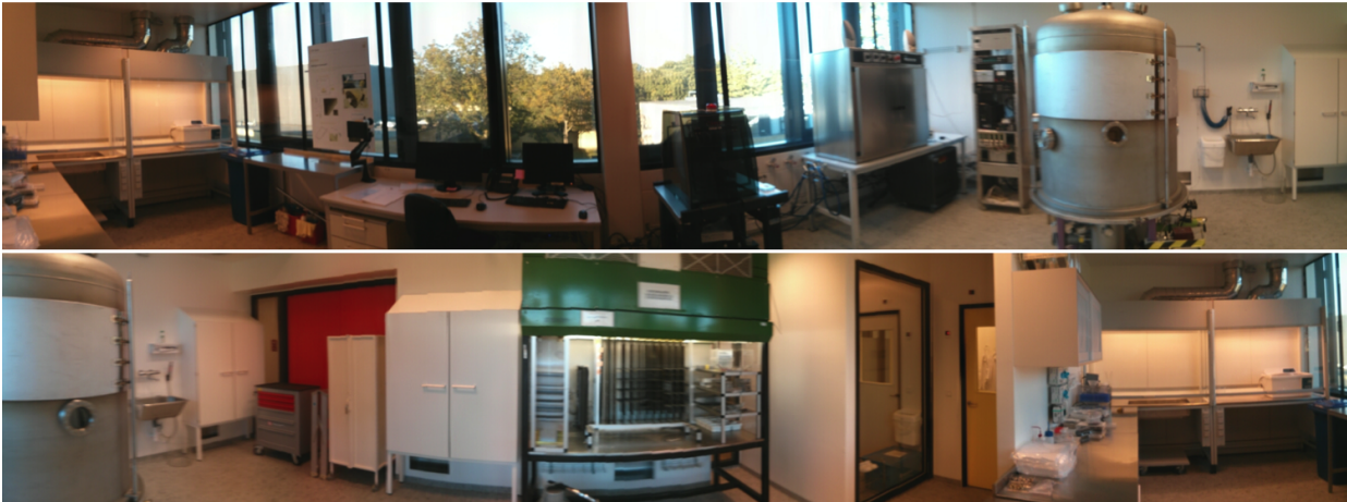
Figure 2.1: Panoramic view of the Multilab coating facility at DTU Space. Top right can be seen the bell-shaped coating chamber.
