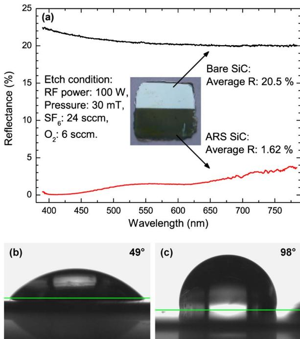
Fig. 2. (Color online) (a) Surface reflectance of the bare and ARS SiC samples measured at near-normal incidence of  $6^\circ$ , inset: photograph of the bare (top half) and ARS SiC (bottom half). Water droplet contact angle measurements on (b) bare SiC ( $49^\circ$ ) and (c) ARS SiC ( $98^\circ$ ).
