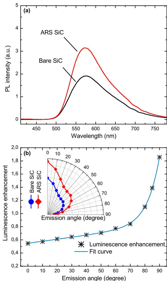
Fig. 3. (Color online) (a) PL spectra of the bare and ARS SiC measured at  $0^\circ$ . (b) Luminescence enhancement of the SiC at different emission angle after introducing the ARS. Inset: spatial emission patterns for both bare and ARS SiC.
