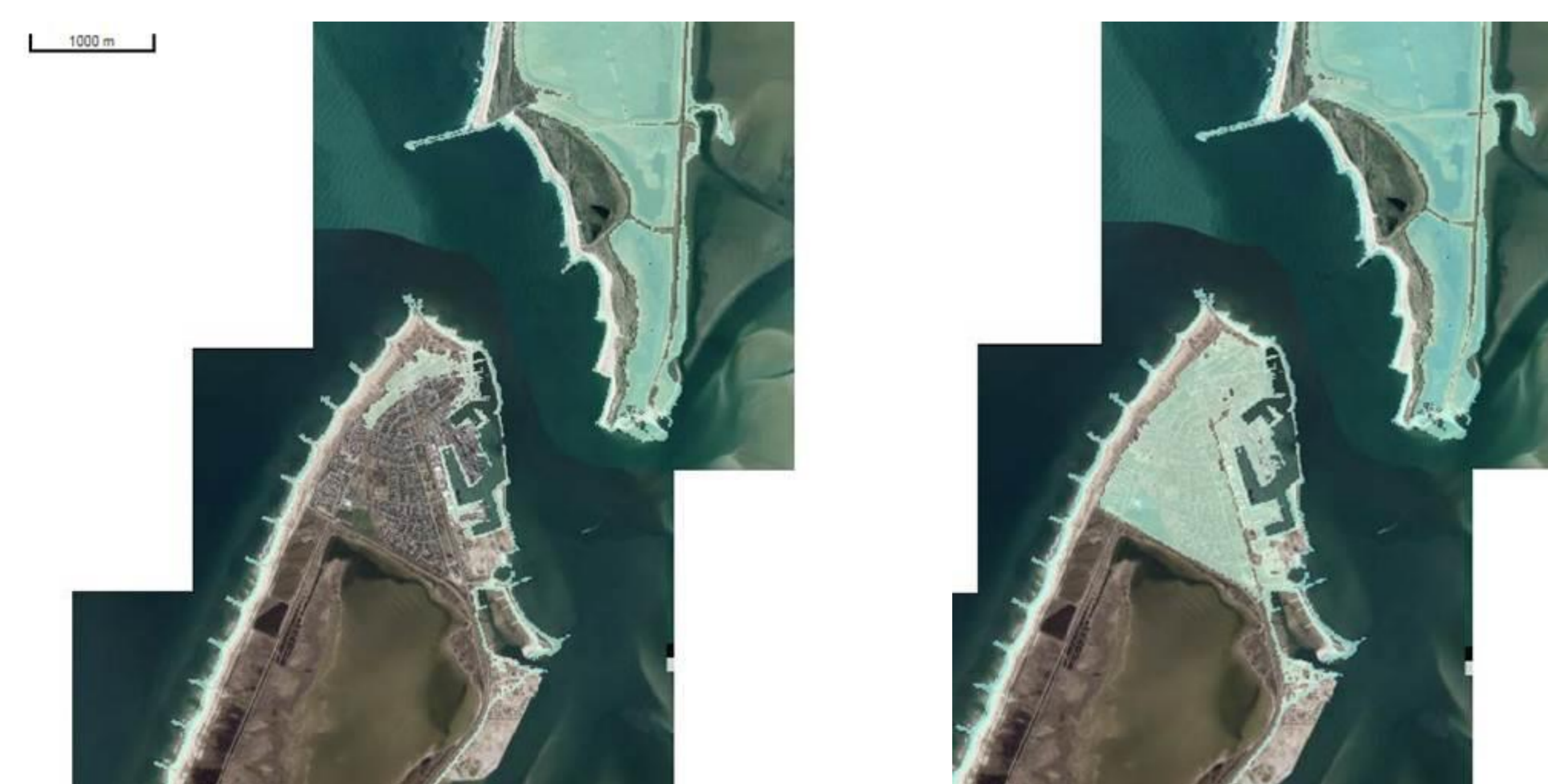
Figure 5. Potential flooding extent from a storm surge at Thyboron Harbor with a return period of 50 years in 2016 (left) and in 2060 including sea level rise and land subsidence.
