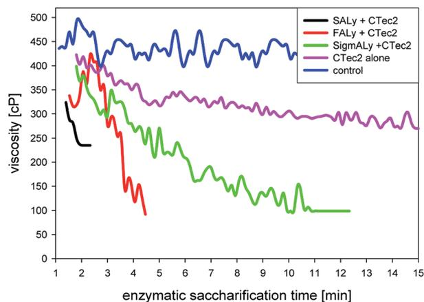
**Fig. 7** Evolution of viscosities at shear rate of 60 rpm over 15 min of enzymatic treatment with Cellic@CTec2 and alginate lyase (SALy, FALy, SigmALy); Cellic@CTec2; and the control without any enzyme addition.
