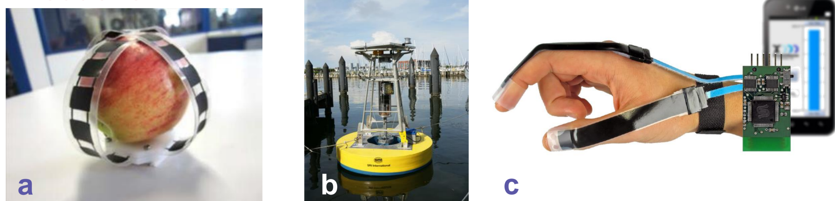
Three modes of application of dielectric elastomer in artificial muscles technology: a) actuator, b) generator, c) sensor
