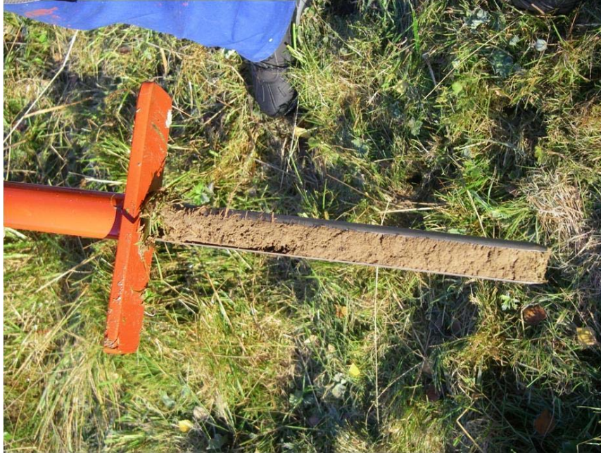
Figure 4: Soil sampler used in RADPAST project. All participants used the same instrument for the sampling work.
