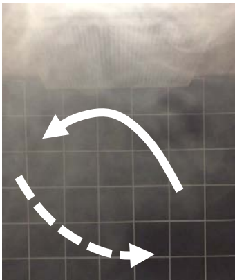
Fig. 4 Seeded smoke occludes fore- and background (frame 1263). Air currents are circular, no clear exhaust stream.
