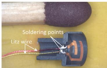
Fig. 3 LDS lines in the RIC connector. [6]
