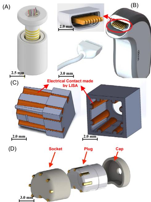
Fig. 4. The conceptual designs of four micro connectors.
