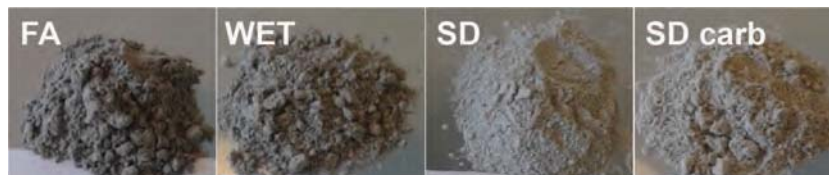
Figure 1: FA and air-pollution control (APC) residues from the incineration of municipal solid wastes: FA (FA from the ESP of an incinerator in Greenland), WET (APC residue from a wet-system in Denmark), SD (APC residues from a semi-dry system), SD carb (carbonated SD sample).
