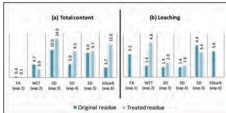
Figure 3: Comparison of mercury total levels and leaching characteristics of MSWI residues before and after ED experiments: (a) mercury concentration (mg/kg dry matter); (b) leached mercury ( $\mu\text{g}/\text{kg}$  dry matter).
