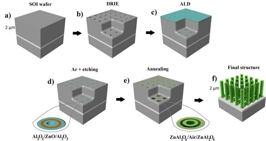
Figure 1. Schematic drawing of the multistep fabrication
