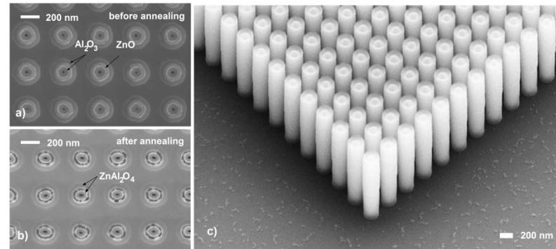
Figure 2. Electron micrograph images. (a) ALD deposition of initial coatings. (b) Temperature induced Kirkendall effect and the formation of  $\text{ZnAl}_2\text{O}_4$  hollow coaxial pillars. (c) Final structure after selective silicon removal.
