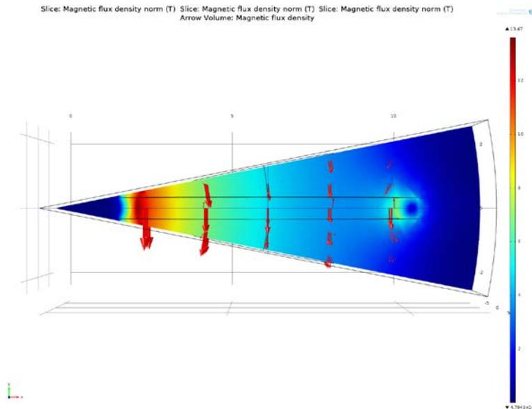
Figure 28. Magnetic flux density of TF coil when  $ITF = 14.5 \text{ A}$  ( $J_{\text{coil}} = 27 \text{ A/mm}^2$ ) resulting in a value of  $B \sim 13.5 \text{ T}$  on the conductors, but a center flux density of  $4.9 \text{ T}$  being lower than the power plant Scenario D with  $5.6 \text{ T}$  [1]. The Cost of Capacity of the coated conductor TF coils is estimated to be  $15 \text{ MEuro/MW}$ .
