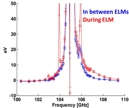
Figure 14. Spectral power density for an NBI heated AUG plasma discharge during an ELM event (in red) and in between ELMs (in blue).
