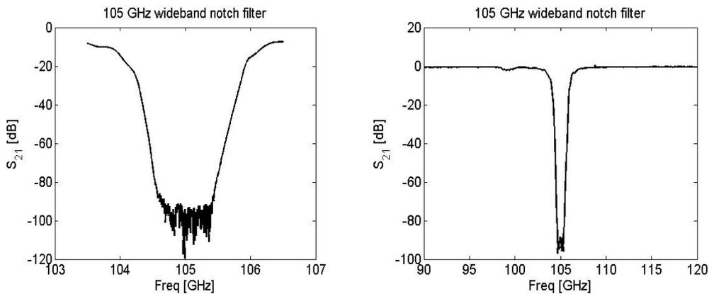
Figure 25. A notch filter with wide rejection made for the ECE group at ASDEX Upgrade. This filter will protect the ECE receiver during piggy-back experiments where the CTS group is also participating.
