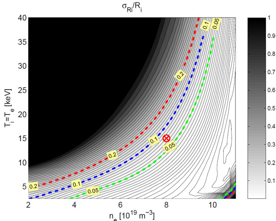
Figure 11. Expected relative uncertainty in measurements of the fuel ion ratio,  $R_i = n_T/n_D$ , on JET a function of plasma density and temperature. The results indicate that reasonable accuracy can be attainable for wide ranges of temperatures and densities, but likely not in so-called hot ion H-modes where the density is kept low in order to achieve very high ion temperatures.
