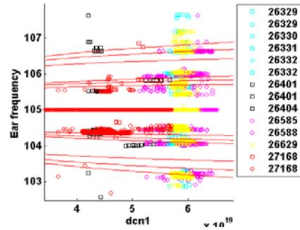
Figure 17. The frequency of the ears is plotted over the central electron density for several discharges. The red lines indicate typical frequency ranges of  $f_{gyr} \pm f_{LH}$  and  $f_{gyr} \pm 2f_{LH}$ .
