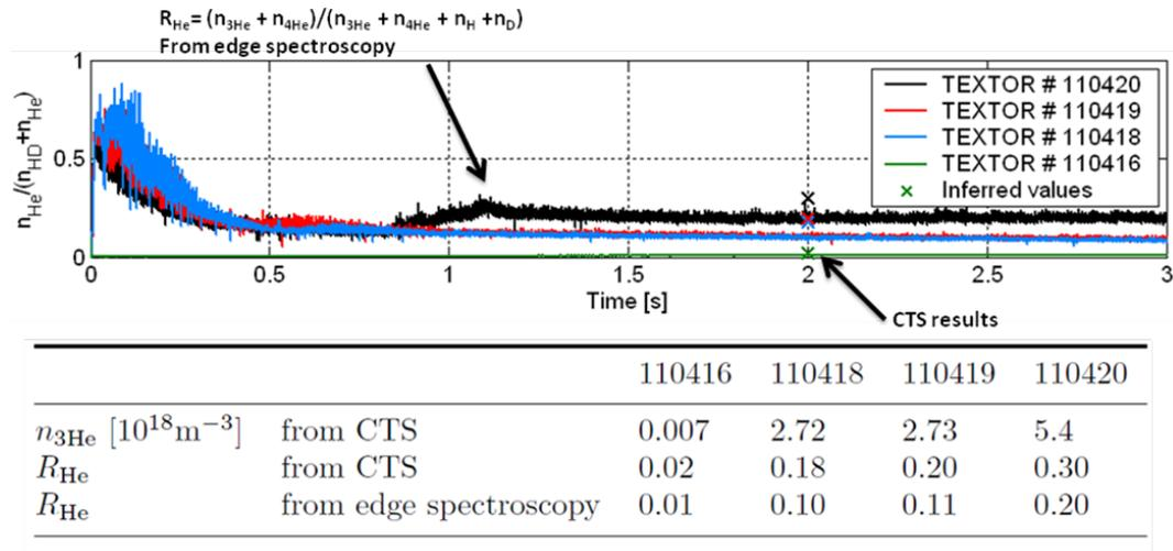
Figure 9.  $^3\text{He}$  densities measured at the plasma edge by CXRS and in the plasma core by CTS. Despite aggressive fuelling with  $^3\text{He}$  during the start-up phase and continuous fuelling in discharge 111420 the plasmas were dominated by recycled hydrogen and deuterium from the vacuum vessel walls. The CTS and CXRS results are similar and show the same trends, and the differences could indicate different plasma compositions in the core and edge regions.
