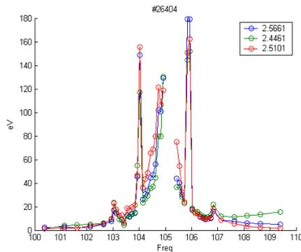
Figure 16. Measurement of very large SPDs at about  $\pm 1$  GHz frequency shift from the gyrotron frequency  $f_{gyr}$  (105 GHz). Typical measurements at 3 different times are shown here. A second set of smaller peaks appears at  $f_{gyr} \pm 2$  GHz
