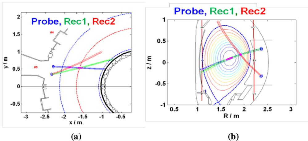
Figure 19. Scattering geometries for the CTS at ASDEX Upgrade, (a) top view (b) poloidal projection. Blue depicts the gyrotron beam, green and red depicts the beams for each receiver as depicted in Figure 18.
