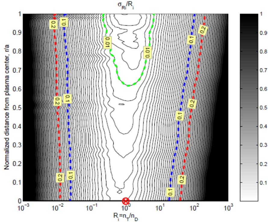
Figure 10. Expected relative uncertainty in measurements of the fuel ion ratio,  $R_i = n_T/n_D$ , in ITER as a function the fuel ion ratio and the position of the CTS scattering volume given as distance from the plasma center normalized by the plasma minor radius,  $a$ . In the plasma core,  $r/a=0$ , the relative uncertainty is within the 20% level on the range  $0.01 < R_i < 40$ . Outside the core this range can be somewhat wider due to the lower temperature there.
