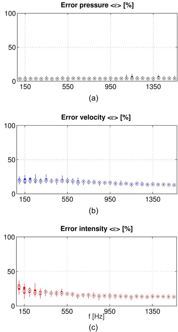
FIG. 6. (Color online) Relative error of pressure, particle velocity, and sound intensity  $20 \log(|\mathbf{x} - \tilde{\mathbf{x}}|/|\mathbf{x}|)$  where  $\mathbf{x}$  is the true field and  $\tilde{\mathbf{x}}$  the reconstructed/estimated field.
