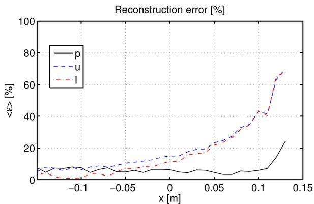
FIG. 7. (Color online) Spatially averaged reconstruction error as a function of position: normalized error over the reconstruction plane for different reconstruction distances from  $x = -20$  cm (forward propagation) to  $x = 0.13$  (back-propagation, just in front of the source).
