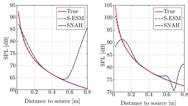
FIG. 9. (Color online) Comparison of methods: true pressure (solid line); proposed S-ESM method (dashed line); SNAH method (dashed-dotted line). Left:  $ka = 0.5$ . Right:  $ka = 2$ .
