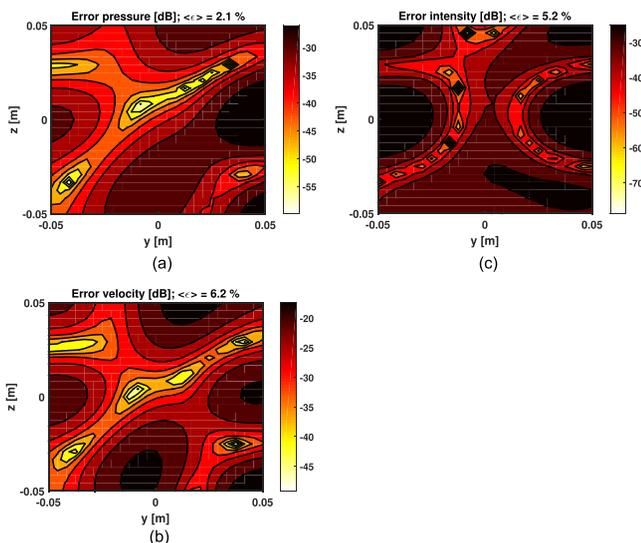
FIG. 5. (Color online) Relative error of pressure, particle velocity, and sound intensity  $20 \log(|\mathbf{x} - \tilde{\mathbf{x}}|/|\mathbf{x}|)$  where  $\mathbf{x}$  is the true field and  $\tilde{\mathbf{x}}$  is the reconstructed field. Also the spatially averaged error is given in %.
