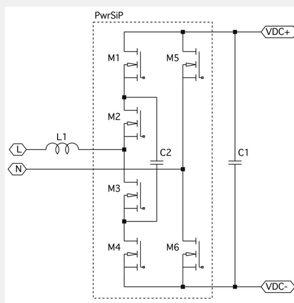
Figure 3. Bridgeless Totem Pole Rectifier with Flying Capacitor
