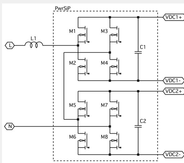
Figure 2. Cascaded Multi-Cell Rectifier
