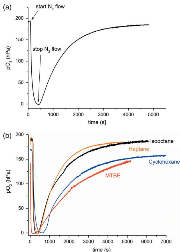
**Figure 3.** (a) Dynamic method for determination of oxygen transfer rates from the headspace to heptane system. (b) Dynamic method for oxygen transfer measurements from isooctane, cyclohexane, MTBE and heptane.
