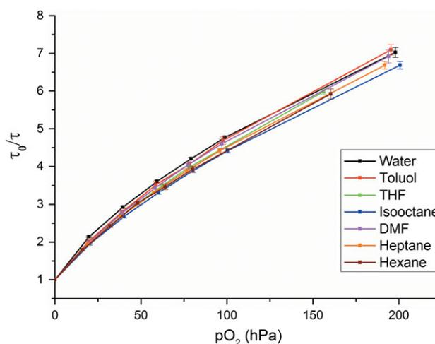
**Figure 1.** Calibration curves of oxygen sensors in different organic solvents at 25 °C.
