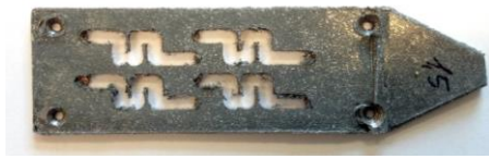
Fig. 1. TinCo 50 plastic plate with the antenna patterns cut along the X axis. Length of each antenna: 30 mm ( N/4 ).
