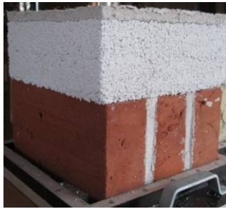
Figure 1: Model of vault construction with insulation mortar; ½ brick thick vault, 100 mm insulation mortar and 10 mm cattle hair reinforced mortar
