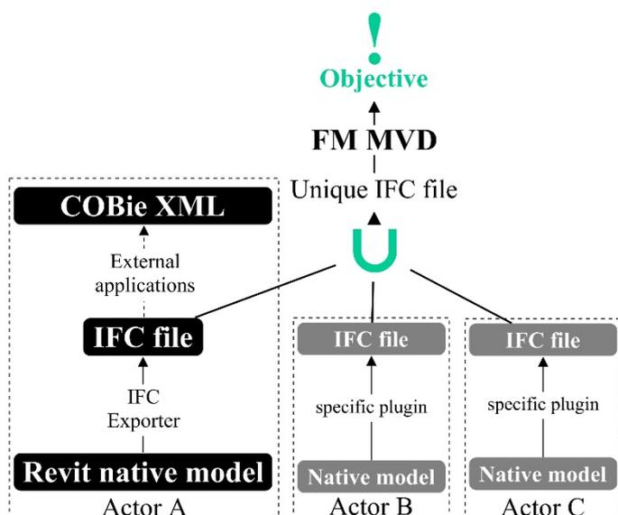
Figure 4. Delivering COBie data using a comprehensive perspective.
