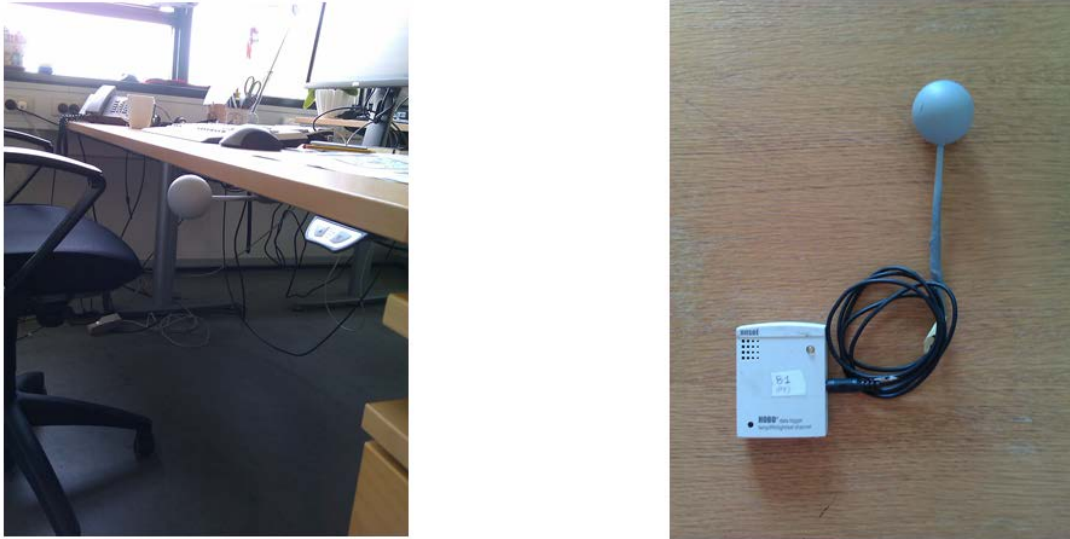
Figure 1 - (Left) Illustrative placement of an operative temperature sensor at a workplace, (Right) A set of grey sphere-shaped sensor and data logger
