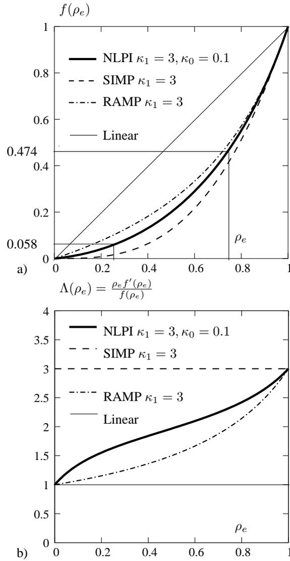
Figure 2: a) The interpolation functions, with the specific values corresponding to  $\rho_e = 0.25$  and  $\rho_e = 0.75$  to be used in Section 7.2. b) The factors for the sensitivity, defined in (19).
