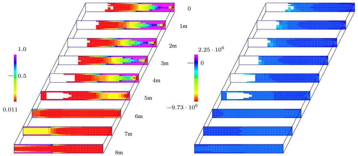
Figure 14: Clamped support, non-linear interpolation with  $\kappa_1, \kappa_0 = 3, 0.1$ , and 25% material. Left the optimized density distribution and right the corresponding distribution of OC values. Linear scales for density and OC values; white for  $\rho_e < 0.011$ .
