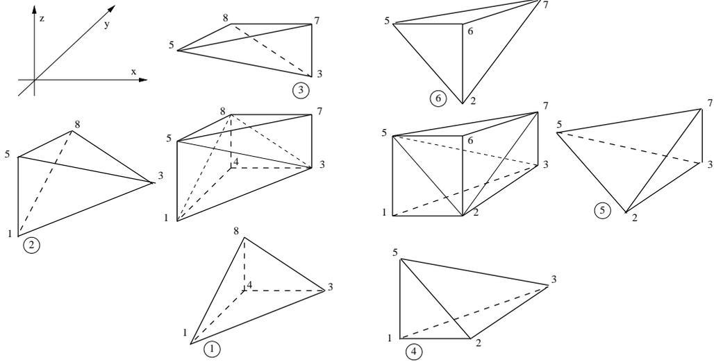
Figure 1: Eight node hexahedron element divided first into two wedges elements and then into six tetrahedra elements, numbered in circles. The numbering of the eight nodes of the hexahedron is also related to the corner nodes of the tetrahedra.
