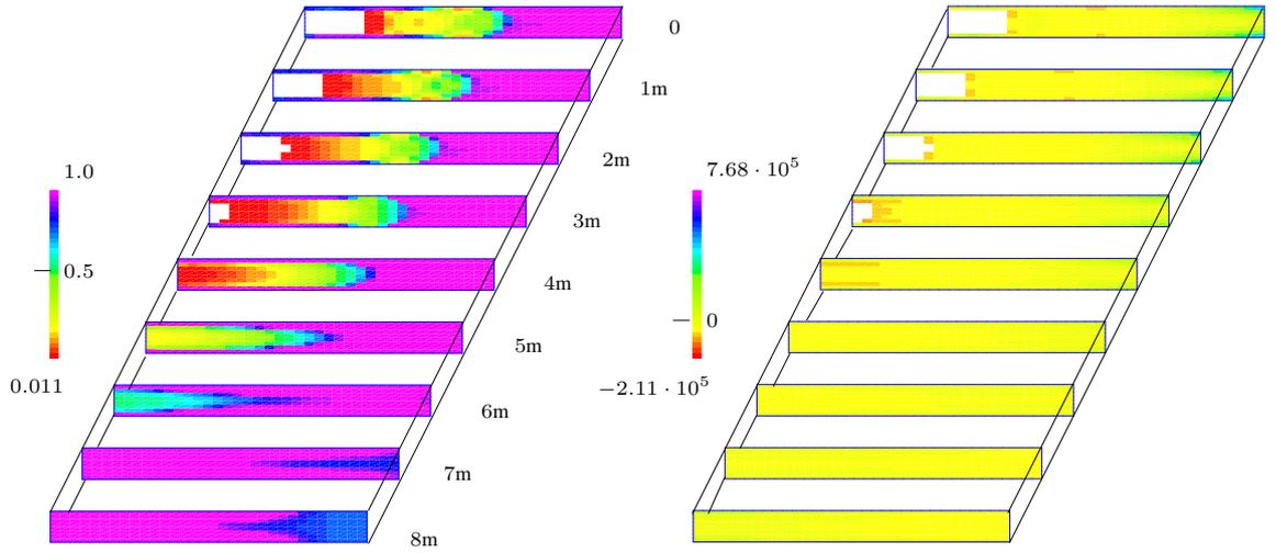
Figure 13: Clamped support, non-linear interpolation with  $\kappa_1, \kappa_0 = 3, 0.1$ , and 75% material. Left the optimized density distribution and right the corresponding distribution of OC values. Linear scales for density and OC values; white for  $\rho_e < 0.011$ .
