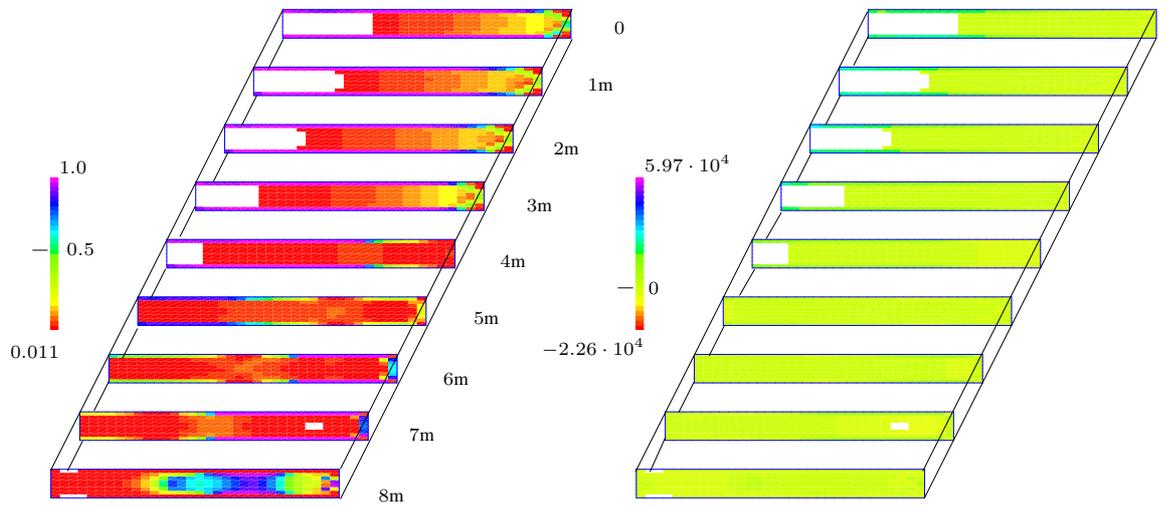
Figure 10: Simple support, non-linear interpolation with  $\kappa_1, \kappa_0 = 3, 0.1$ , and 25% material. Left the optimized density distribution and right the corresponding distribution of OC values. Linear scales for density and OC values; white for  $\rho_e < 0.011$ .
