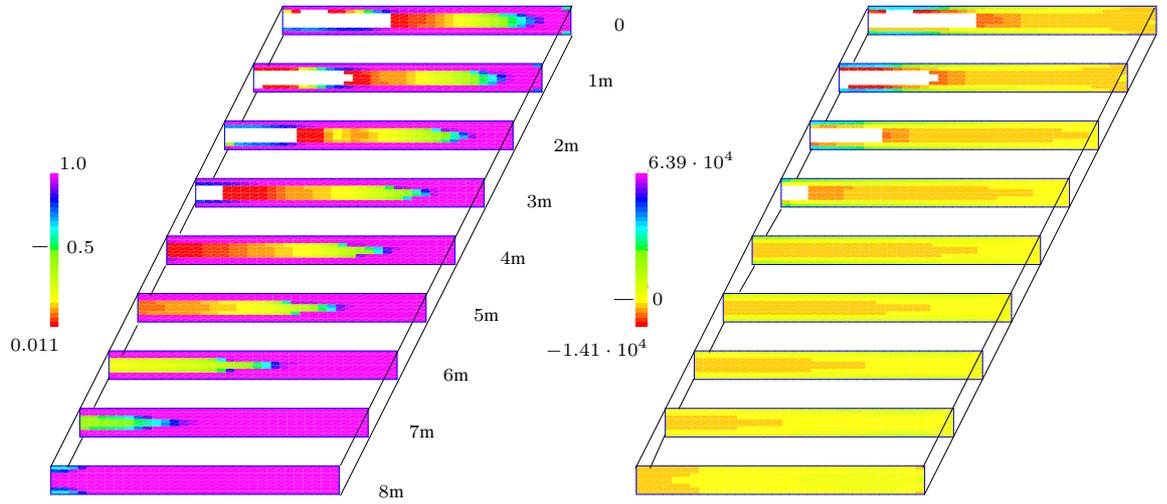
Figure 9: Simple support, non-linear interpolation with  $\kappa_1, \kappa_0 = 3, 0.1$ , and 75% material. Left the optimized density distribution and right the corresponding distribution of OC values. Linear scales for density and OC values; white for  $\rho_e < 0.011$ .
