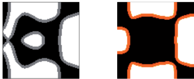
Fig. 13 Electrode pattern that isolates the 6th mode among the first 20 modes in a plate fixed at its left side; (left) the gap is imposed a posteriori; (right) the gap is considered in the formulation.
