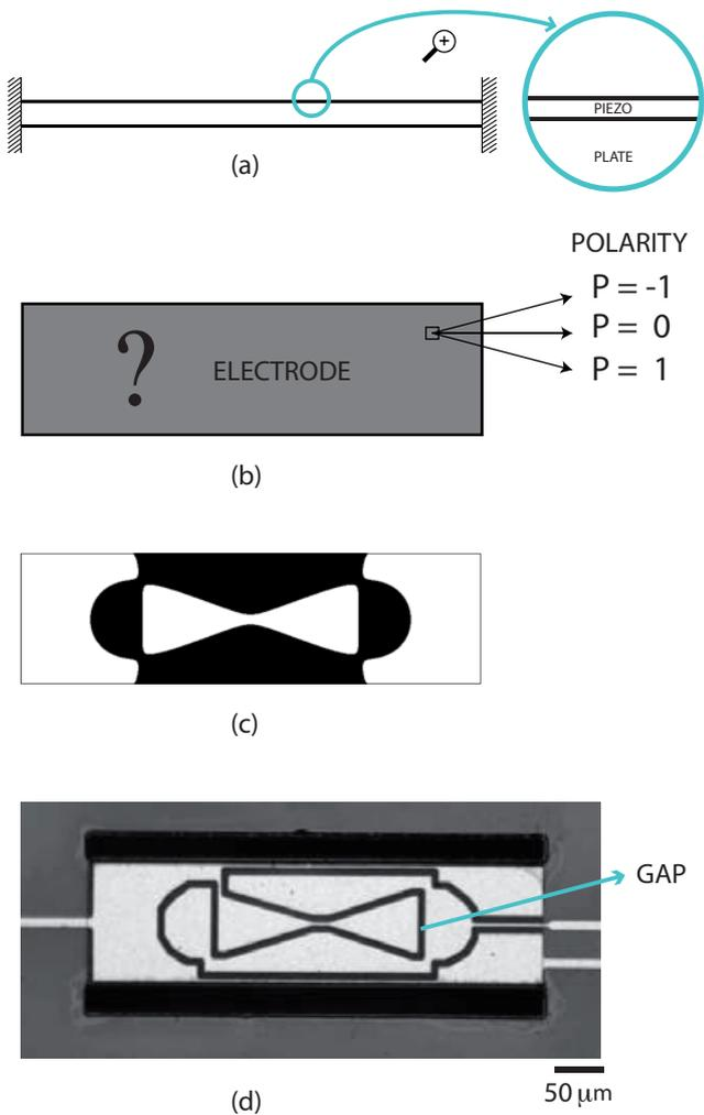
**Fig. 2** (a) Side view of a micro plate of 680  $\mu\text{m}$  in length and 200  $\mu\text{m}$  in width clamped at its both extreme sides; (b) Top view of the design domain (electrode); (c) Electrode profile that isolates the first mode from the first 14 out-of-plane modes. Black and white phases denote regions with opposite polarity; (d) Manufactured design with a gap-phase of width  $w_{\text{gap}} = 5 \mu\text{m}$ . This example has been extracted from Sánchez-Rojas et al. (2010).
