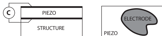
Fig. 1 Schematic diagram of a piezoelectric transducer; (left) cross section of a structure with a piezo layer surface bonded; (right) top view of the surface electrode.
