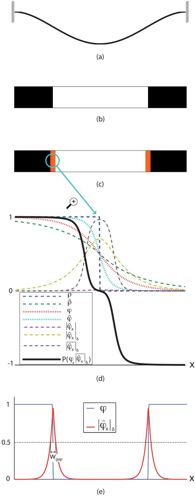
**Fig. 4** (a) First mode of a clamped-clamped beam of  $L$  length; (b) Electrode profile that maximizes this shape, where black and white phases mean regions with opposite polarity; (c) The same on including a gap-phase of width  $w_{gap} = 0.03L$  in each interface; (d) Interpolation function for the electrode profile with underlying two-step filtered fields; (e) On how the gap width is derived.
