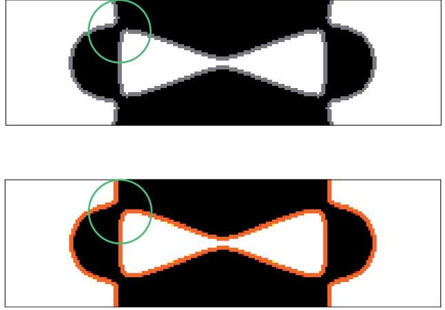
**Fig. 9** Electrode pattern that isolates the 1st mode among the first 14 modes in a plate clamped at its both extreme sides; (top) the gap is imposed a posteriori; (below) the gap is considered in the formulation. Green circle represents where small differences occur between the designs.
