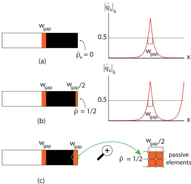
**Fig. 5** (a) Half electrode profile of the previous example on using null Neumann boundary conditions; (b) Same with Dirichlet boundary conditions; (c) Same with Dirichlet boundary conditions and a passive area.
