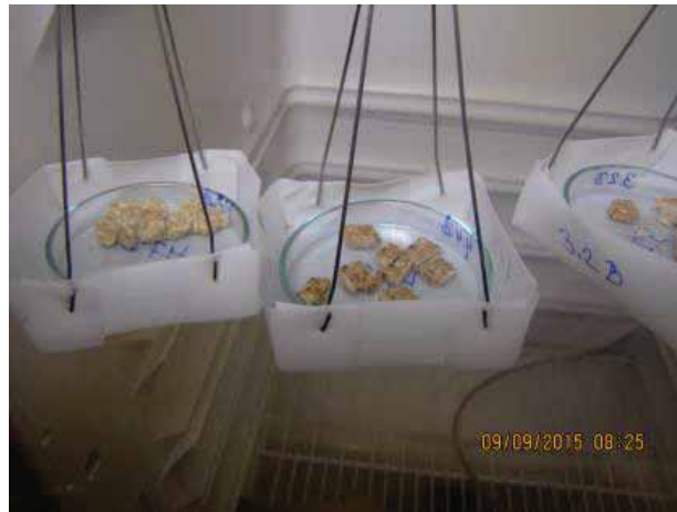
Figure 10: Specimens in the petri glass dishes placed in baskets.
