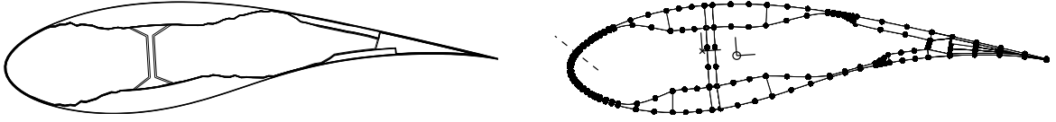
Figure 12: (a) Schematic of rotor blade cross-section (b) Discretization using 45 internally layered elements.
