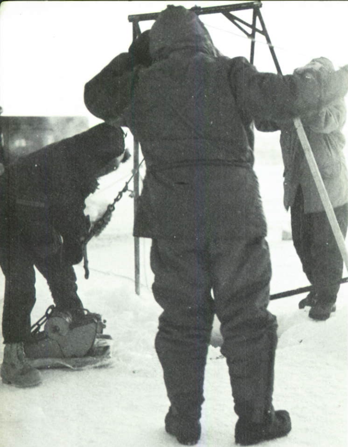
Bottom sampling is seen on the ice placed on a plastic sheet to avoid contamination (middle left). The snowmobile was used for transportation as well as for hoisting the grab.
