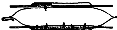
Figure 3. The intensity of beta-radiation originating from radioactive elements embedded in a sherd is measured by means of the phosphor \text{CaSO}_4:\text{Mn} cemented to a metal plate.
