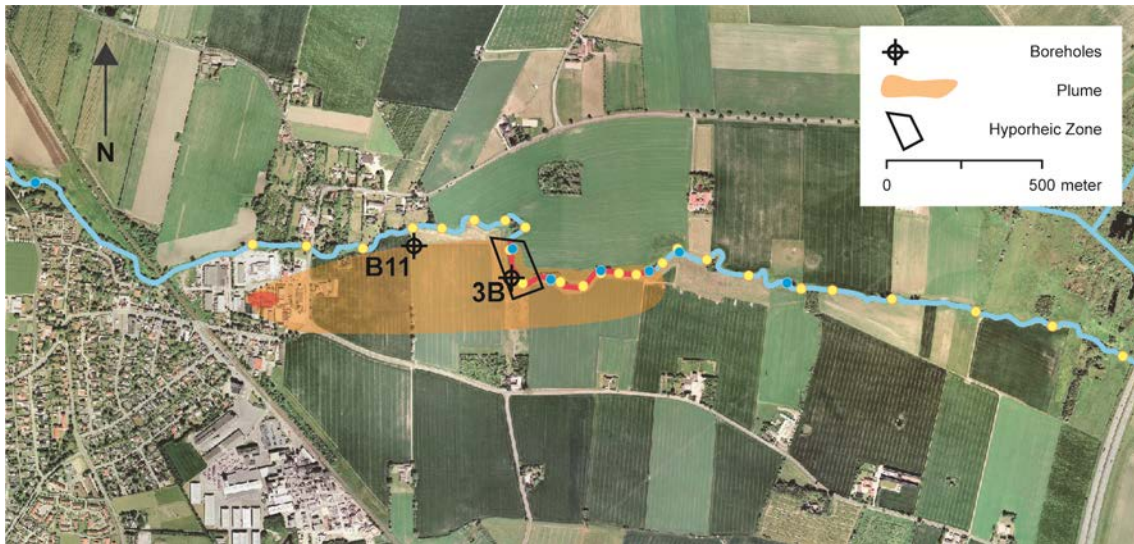
Figure 1: Propagation of the TCE contaminant plume and impacted stream section at the Lille Skensved site. Also shown are the measurement locations in the stream (yellow dots) and stream bed (blue dots), the location of the remediation well (B11) used for pump and treat, and the location of the well in the hyporheic zone (3B).
