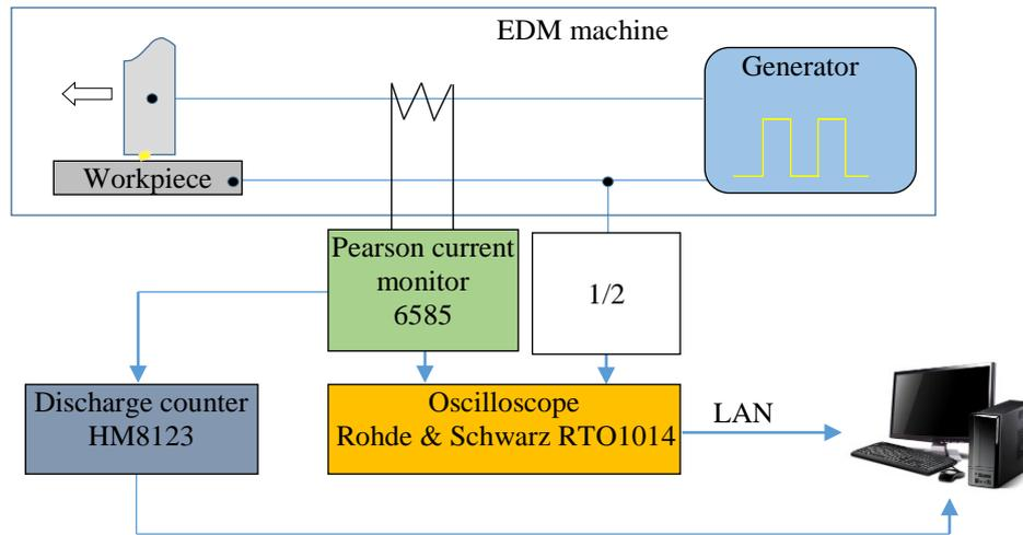
Fig. 1 A schematic diagram for the experimental procedure
