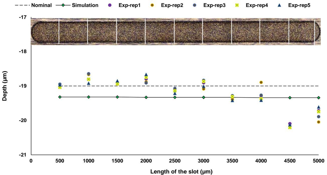
Fig. 19 The nominal, simulated and experimentally measured depths at TWD =  $3.43 \mu\text{m}^3$  (number of layers machined = 19)
