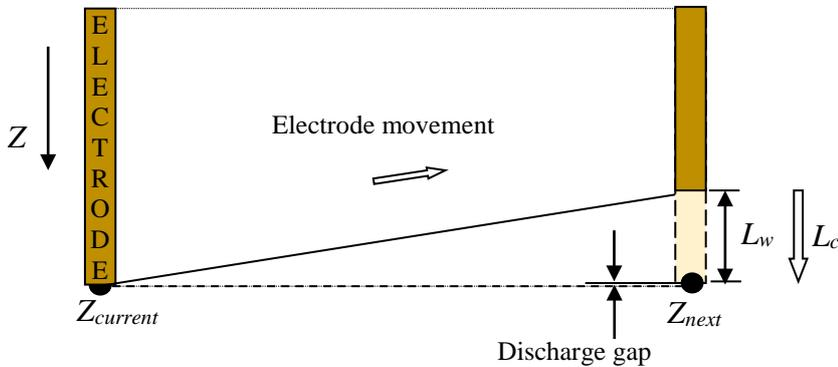
Fig. 5 Illustration of the electrode wear compensation method using TWD method
