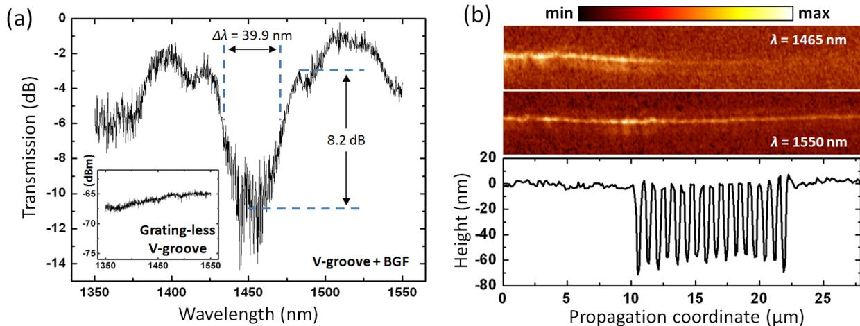
Fig. 2. (a) Transmission measurement of a V-groove containing a 16-period BGF. Inset: reference transmission through a similar but grating-less V-groove. (b) NSOM measurements for two different wavelengths ( $\lambda = 1465$  nm and  $\lambda = 1550$  nm) showing the spectral rejection for the former. An AFM cross-section shows the corresponding profile along the propagation direction.
