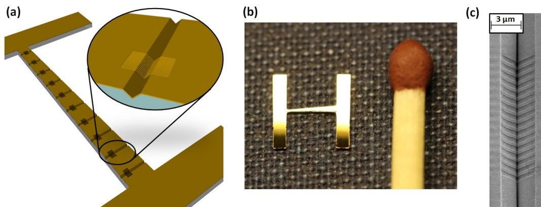
Fig. 1. (a) Illustration of a device with zoom-in of a V-groove containing a Bragg grating filter. (b) Photograph of a fabricated device beside a common match. (c) Scanning electron micrograph of a fabricated V-groove with 16-period Bragg grating filter.
