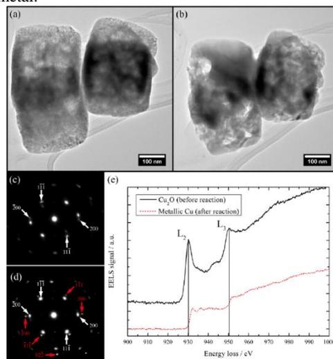
**Fig. 1** Bright-field images, electron diffraction and Electron energy-loss spectra showing the photodegradation of cuprous oxide under optical illumination in an aqueous environment.
