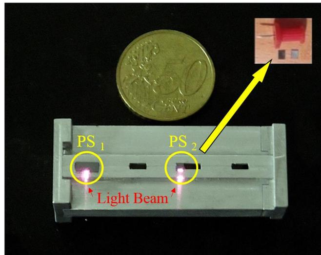
Fig. 1. Optically-controlled reconfigurable slotted-waveguide antenna developed for the experiments. In the up right corner a photoconductive switch and its integration to the reconfigurable antenna is presented
