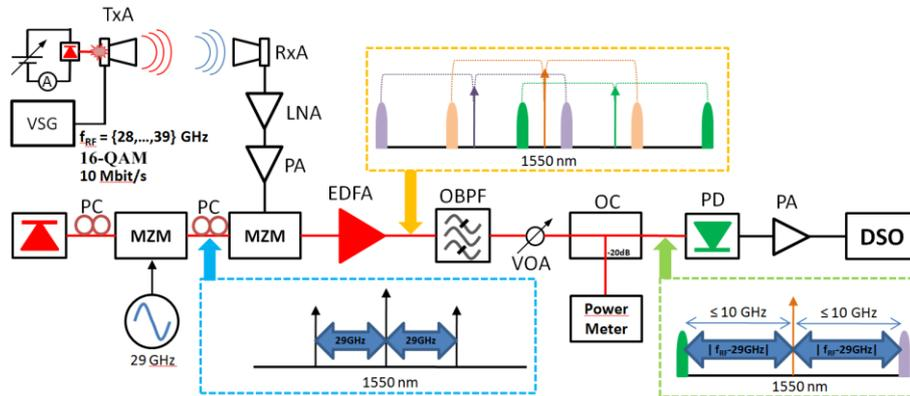
Fig. 5. Experimental setup including the photonic downconversion stage. VSG: vector signal generator, CS: Current Source, TxA: transmitting antenna, RxA: receiving antenna, PC: polarization controller, MZM: Mach-Zehnder modulator, LNA: low noise amplifier, PA: power amplifier, EDFA: Erbium doped fiber amplifier, OBPF: Optical Band Pass Filter, VOA: variable optical attenuator, PD: photo detector, DSO: digital storage oscilloscope; LO: local oscillator.
