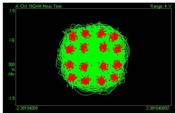
Fig. 6. Constellation of 16-QAM with  $EVM_{RMS} = 3.09\%$  for 38 GHz wireless transmission with photonic downconversion.
