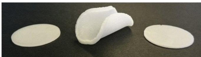
Fig. 9 Images of a 25 mm in diameter and 1 mm thick sample, G40_S184, before the absorption experiment, after absorption and after drying, respectively.
