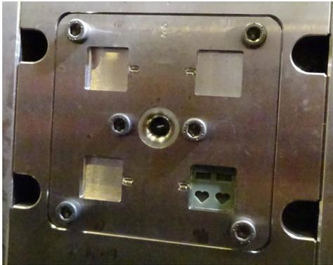
Fig. 3. Single insert in the IM machine before the first shot. [15] (used with permission)
