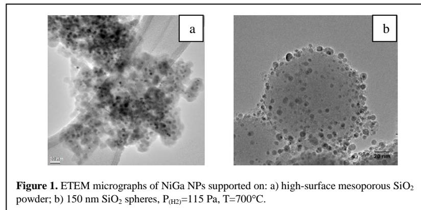
**Figure 1.** ETEM micrographs of NiGa NPs supported on: a) high-surface mesoporous SiO<sub>2</sub> powder; b) 150 nm SiO<sub>2</sub> spheres, P<sub>(H<sub>2</sub>)</sub>=115 Pa, T=700°C.
