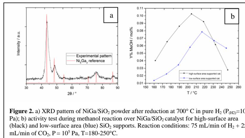
**Figure 2.** a) XRD pattern of NiGa/SiO<sub>2</sub> powder after reduction at 700°C in pure H<sub>2</sub> (P<sub>(H<sub>2</sub>)</sub>=10<sup>5</sup> Pa); b) activity test during methanol reaction over NiGa/SiO<sub>2</sub> catalyst for high-surface area (black) and low-surface area (blue) SiO<sub>2</sub> supports. Reaction conditions: 75 mL/min of H<sub>2</sub> + 25 mL/min of CO<sub>2</sub>, P = 10<sup>5</sup> Pa, T=180-250°C.
