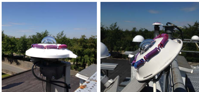
Figure 4. Pictures of the heating elements used to evaporate moisture from the glass dome of pyranometers.
