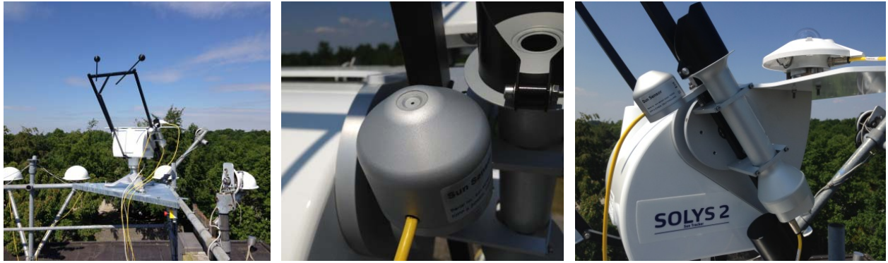
Figure 6. The SOLYS 2 tracker. On the top mounting plate, the pyranometer that measures the diffuse irradiance can be seen. On the left side of the tracker, the solar sensor and the pyrheliometer that measured the beam normal irradiance can be seen.
