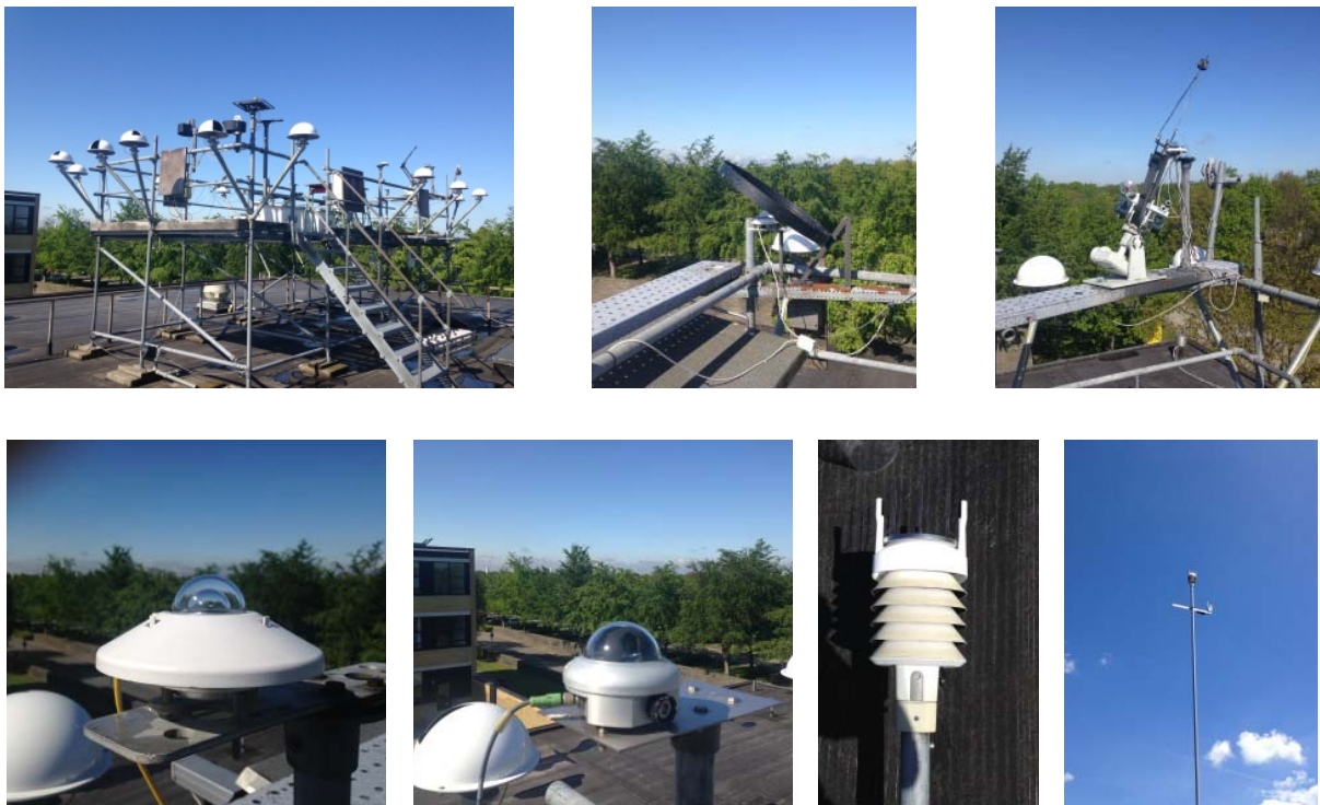
Figure 1. Pictures of the solar radiation measurement station before upgrade and renovation. Top left: Measurement equipment. Top middle: Shadow ring. Top right: the old tracker (Eppley). Bottom left: Pyranometer, type CMP 11 from Kipp and Zonen. Bottom middle left: Sunshine pyranometer, type SPN1. Bottom middle right: Weather station, type Vaisala WTX520 from Oyj in Finland. Bottom right: Vaisala mounted 6 meter above the roof of building 119.
