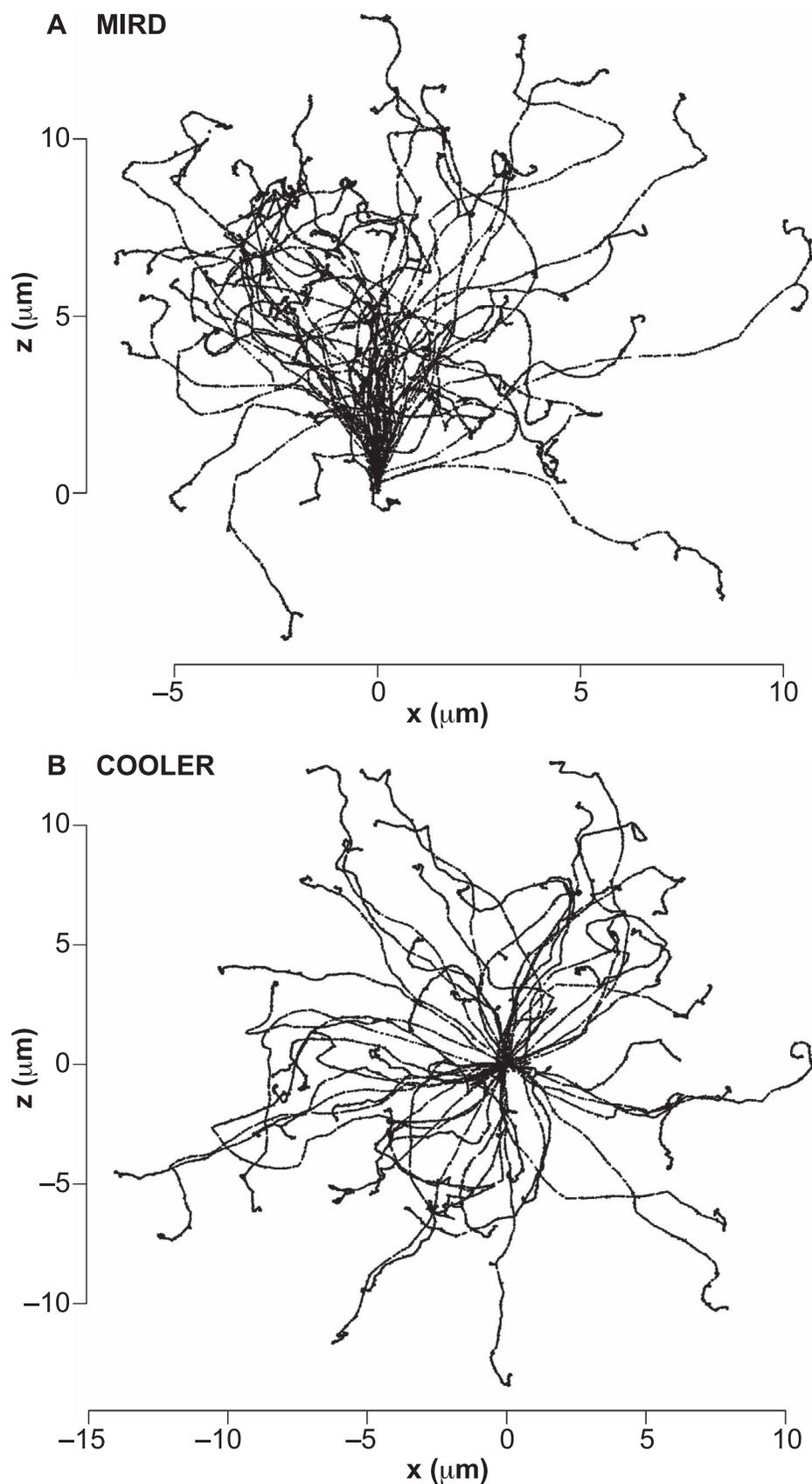
**FIG. 1.** 30 keV electron tracks generated in liquid water using the Monte Carlo code PARTRAC. Panel A: Experimental setup adopted by Cole (20) and MIRD (1). Panel B: The particle emission mode used in this work to determine the deposited energy against distance interrelations.
