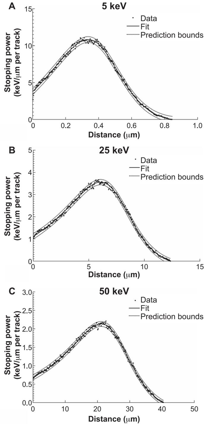
**FIG. 4.** Equation (9) to fit PARTRAC energy-deposition data (dots) as a function of distance is indicated by the black line, together with its 95% confidence bounds for three different initial energies, 5, 25 and 50 keV electrons (panels A–C, respectively)
