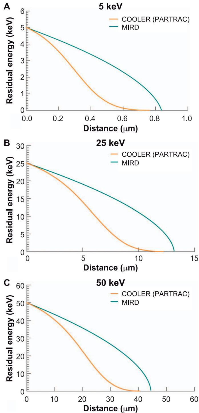
**FIG. 5.** Residual energy versus traveled linear distance relationships, calculated from COOLER (PARTRAC) energy deposition data tables (orange lines) and with the formalism adopted by MIRD (blue lines), are shown for 5, 25 and keV electrons (panels A–C, respectively).
