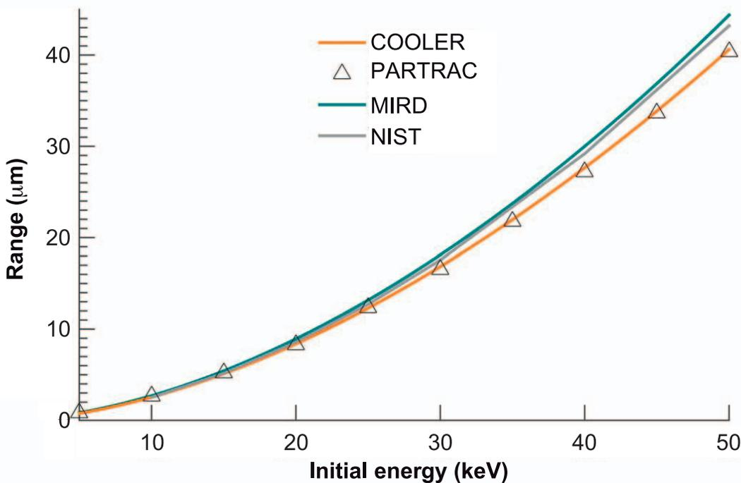
**FIG. 3.** Energy versus range dependence obtained by Cole (20), adopted by MIRD (1) and shown in Eq. (5) is indicated by the blue line. Such a relationship is in good agreement with NIST (46) range values, which are given only for energies above 10 keV (gray line). COOLER range values are shown in orange and determined by Eq. (8). Triangles represent PARTRAC simulated range values.
