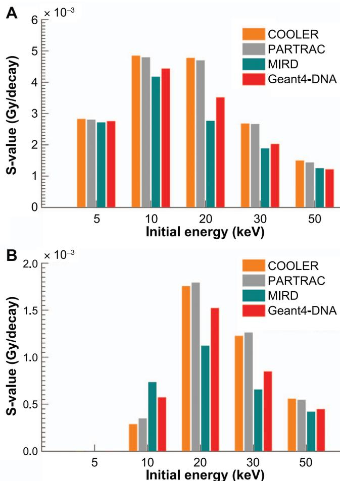
**FIG. 8.** A comparison of cellular S-values for electron emitters, obtained with COOLER (orange), PARTRAC (gray), MIRD (blue) and Geant4-DNA (red) is shown. Results with Geant4-DNA were obtained from (53) for the  $N \leftarrow N$  (panel A) and  $N \leftarrow CS$  (panel B) cases, with a spherical cell geometry (cell radius 5  $\mu\text{m}$ ; nucleus radius 4  $\mu\text{m}$ ). COOLER/PARTRAC results were obtained from dedicated calculations with the same cell model.
