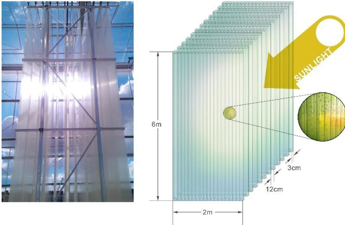
Figure 9. Photo of light dilution design in Ecoduna PBR, where each panel can be seen receiving direct sunlight (*left*), design schematic of Ecoduna PBR with dimensions; *callout* demonstrating microalgal growth, aeration bubbles, and the effect of sunlight reaching the panel (*right*). The arrow represents direct sunlight reaching one face of every panel as the module tracks sunlight.
